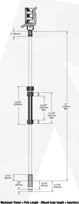
Maximum Travel = Fore Length - (Mount body fengul + Insertion) = 57.00" - (14.58 + 2.01 + 2.48) = 37.93" Minimum Pole Length = Mount body length - Insertion = 14.48" + (2.01 + 2.48") = 19.07" = 20.00"
