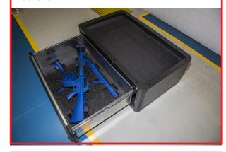
4. (2 person job) Place Cabinet in the rear of vehicle and set into place. The holes in the base should line up with factory mount locations and fasten into place.
