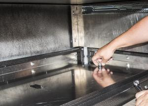
5. Reinstall drawer into CopBox Cabinet. make sure slides fit into roller bearing case securely without binding up.
