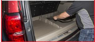
2. Remove factory cargo screws and pull out factory cargo floor.
