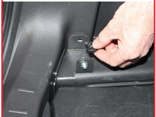
5. (2 person job) Slide CopBox into rear of SUV and slide front lip into the front z-rail mount. Secure the rear with CTECH thumb screws.
