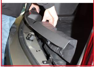
4. \*Spare tire access models only\* Remove factory hook from side panels, install right and left gas shock bracket using factory hook.
