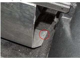
4. Install front mounting bracket with supplied hardward into the nut inserts and Mopar supplied hardware for the 4 seat studs towards the passenger compartment.
