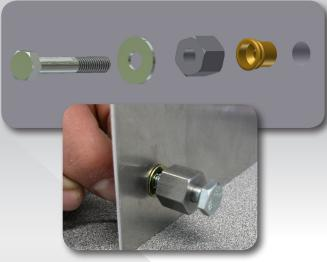
7.Thread nut insert on to hex bolt – tooling compression nut assembly. Nut insert flange should contact machined lip on tooling compression nut.
