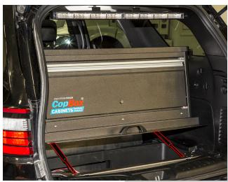
6. Set CopBox Cabinet down and insert CTech knobs to secure rear of CopBox Cabinet.
