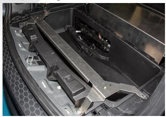
3. Remove factory clip from storage container in floor and replace with supplied nut insert. Please see nut insert procedure for installation instructions. (mount panel will not be installed at this point)
