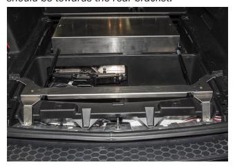
6. Set CopBox Cabinet into vehicle and slide QuickLink front lip on the CopBox Cabinet into the Z Rail on the front bracket.
