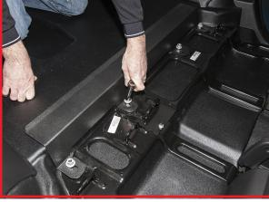
3. (2 person job) Place CopBox Cabinet in the rear of cargo area in SUV and slide forward into Z-Rail front mount. Line up rear holes in base.
