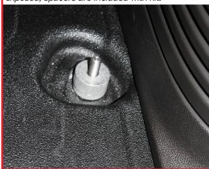
2. Flip up rear seats and remove factory nuts. Place front Z-Rail mounting brack on the seat stud and reinstall factory nuts.
