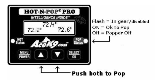
Activate the K9 Door Popper® by pressing the button on the Remote Control Transmitter, or from the Hot-N-Pop® Pro Control Head by pressing BOTH the ▲ and ▼ keys simultaneously. When the door popper is activated the door being popped is unlocked, followed by the latch releasing to open the door. Note the latch is released 2 times in case of obstruction to the door or latch. *Note: if on by arming is selected* pressing the [OK] Button Arms the door popper until the vehicle is put in gear again.
