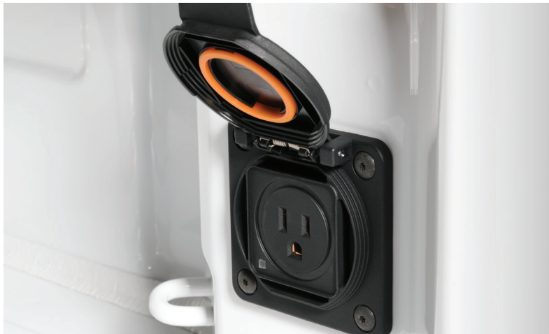
Standard 120-volt power outlet in bed
